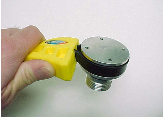
STEP 7A- HR STYLE JACKS WILL USE A PISTON WHICH REQUIRES A STRAP WRENCH TO REMOVE
